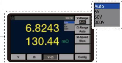
High voltage battery testing up to 1000 V
